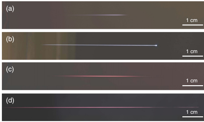
FIG. 6. (Color online) Photographs of the seed filaments and smooth densified plasma channels in argon (two top panels) and helium (two bottom panels). A 40-fs-long, 1.5 mJ igniter pulse is used in the case of argon. The photograph of the seed filament in this case is integrated over 300 laser shots (a). The densified plasma channel in argon remains smooth and continuous as long as the intensity of the nanosecond heater pulse remains under 6 \times 10^{10} W/cm 2 (b). This image is integrated over ten laser shots. In the case of helium, the densified channel is smooth over the entire range of parameters of the igniter and heater pulses attainable in our experimental setup. For example, the dilute seed filament generated by 500-fs-long, 15 mJ igniter pulse in helium is shown in (c). This image is integrated over 100 laser shots. A single-shot image of the channel that is densified through the application of the nanosecond heater pulse with the peak intensity of 2.4 \times 10^{11} W/cm 2 is shown in (d).
